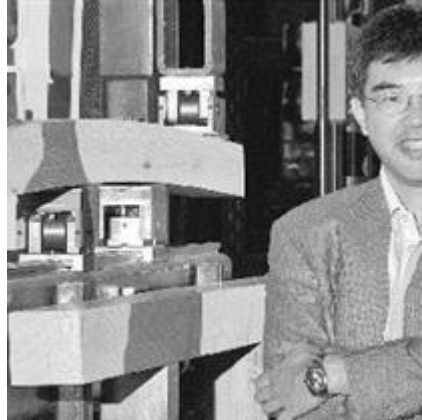
CREDIT: Ian Smith, Vancouver Sun UBC timber engineering professor Frank Lam shows a piece of hemlock (top) under a 2,268-kg (5,000-pound) load.
